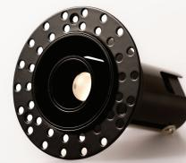
The plaster-in FollowMe.P spotlight allows the user almost complete directional control. The adjustable cylindrical fitting can point in a 355° horizontal range, or, if a 90° vertical spotlight is desired, it can recess back into its fitting to sit flush against the ceiling.
